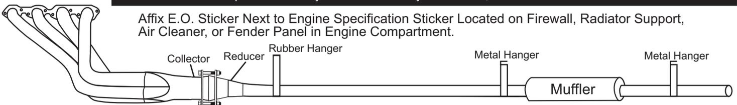
Affix E.O. Sticker Next to Engine Specification Sticker Located on Firewall, Radiator Support, Air Cleaner, or Fender Panel in Engine Compartment.
