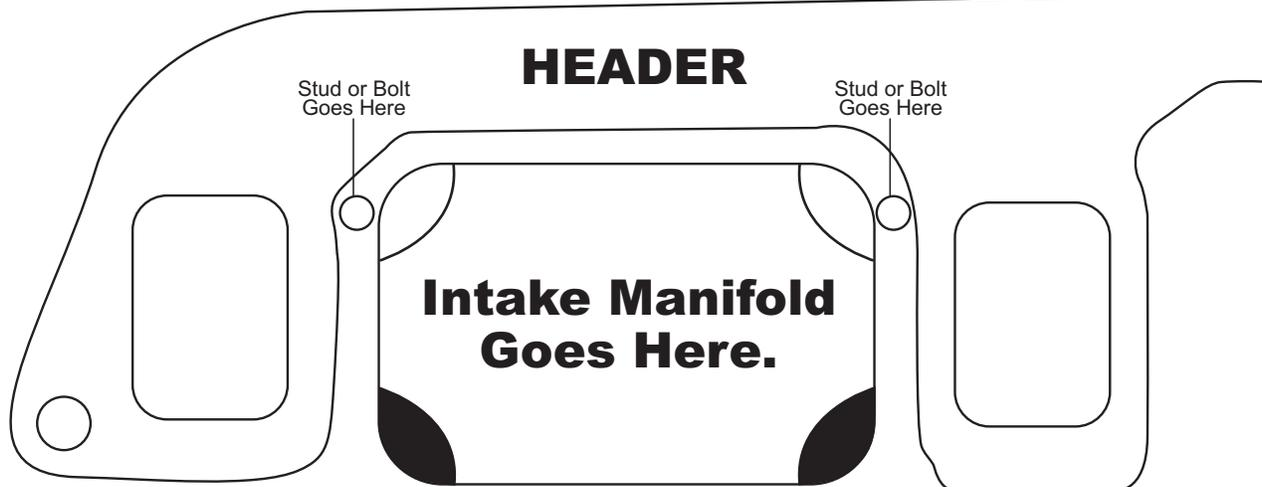
If spacer is too long it may need to be cut to adjust difference in height between intake manifold and header head flange. (If minimal amount of spacer remains, may need to use mill washer, cut 1/3 washer away to use as spacer.)
