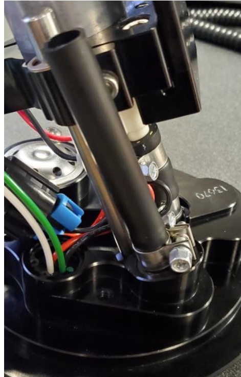
Fig 2: 3-3/8" section of return tube installed on return barb and retained with 12mm clamp
