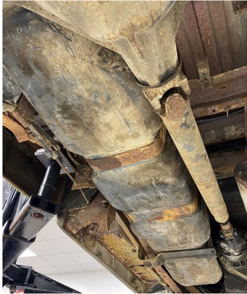
Figure 2 – 74-80 Dodge D100 Fuel Tank
