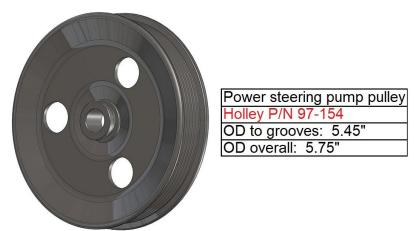
WARNING! Smaller power steering pulleys, such as a 97-154 can rotate the pump beyond recommended RPMs. To correct this, a 25% under-dive balancer should be used if choosing a pump pulley smaller than 6" OD.
