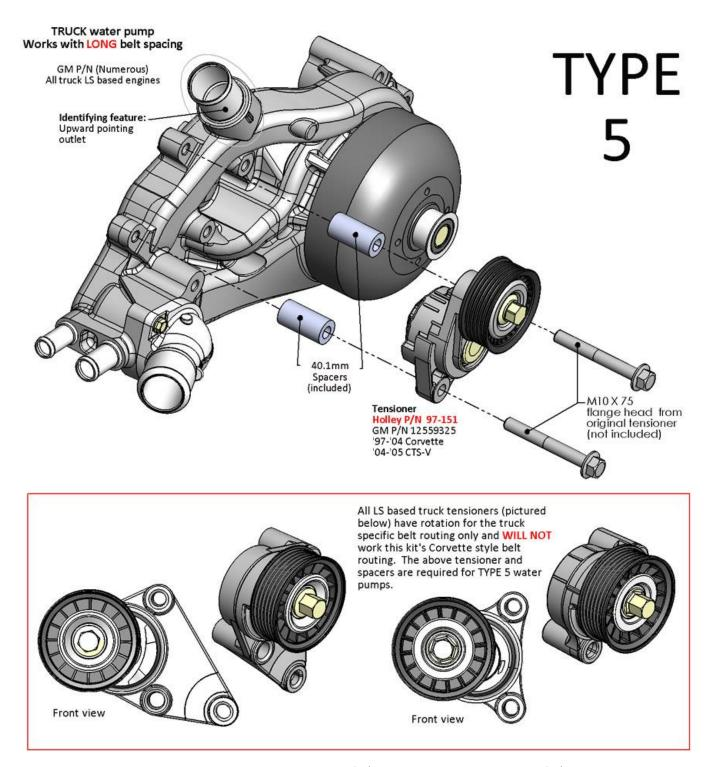
**NOTE:** Torque M8 bolts to 18 ft./lbs. and M10 bolts to 36 ft./lbs.
