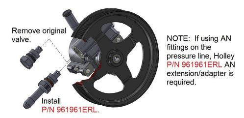
There are several pulleys that will fit the pump, but some do not have the correct belt alignment for this application. See applicable service manual for pulley installation procedures.
