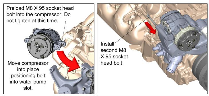
**NOTE:** After assembly torque M8 bolts to 18 ft./lbs.
