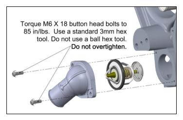
**WARNING:** Do not plug all heater passages. For safe LS/LT engine start up cooling this path must stay open. If not utilizing a heater core, install a jumper hose between the two barbs.
