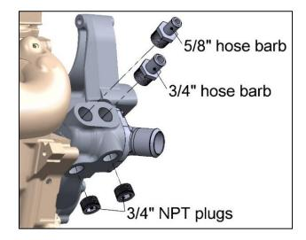
**Configurations:** On some swap applications there is not clearance for side heater hose outlets. There are optional bottom outlets for these applications.
