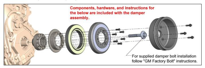
**HELPFUL HINT:** The above parts have a tight slip fit if aligned perfectly before assembly. If the aluminum pulley does not slip in the hub bore, the pulley can be placed in a freezer for 3 hours minimum. Remove and immediately install. Make certain the three pulley holes align to the hub while frozen because after the pulley warms you will likely not be able to rotate it in the hub.
