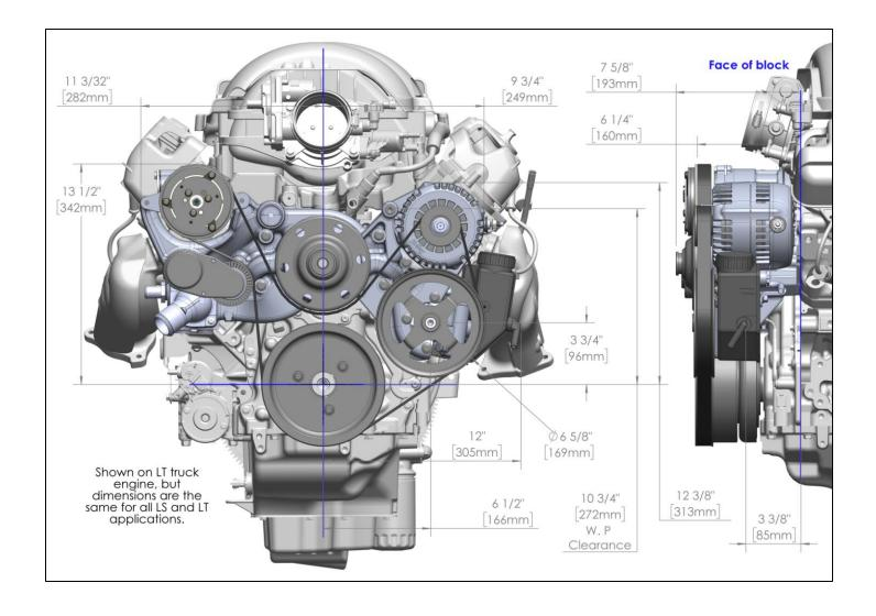
**IMPORTANT NOTE IF PAINTING COMPONENTS:** The alternator and A/C compressor ground through the water pump manifold. If painting or coating the manifold, the mating surfaces must all be bare metal allowing a ground path from the accessories' mounting feet to the engine block and ultimately the negative terminal on the battery.
