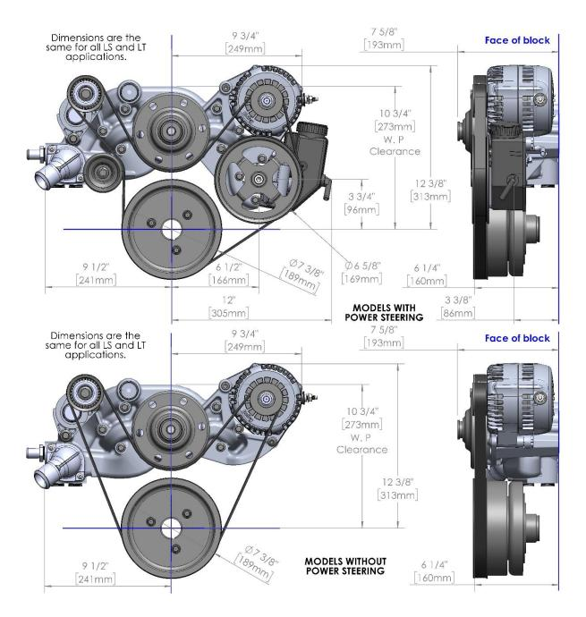
**IMPORTANT NOTE IF PAINTING COMPONENTS:** The alternator and A/C compressor ground through the water pump manifold. If painting or coating the manifold, the mating surfaces must all be bare metal allowing a ground path from the accessories' mounting feet to the engine block and ultimately the negative terminal on the battery.
