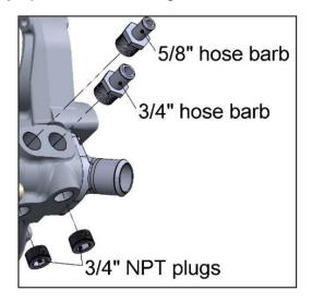
**Configurations:** On some swap applications there is not clearance for side heater hose outlets. There are optional bottom outlets for these applications.
