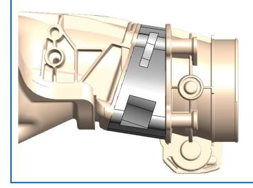
NOTE: The angle adapter is required when using an LT car style intake to prevent interference from the downward facing throttle body. See included instructions for installation procedures.
