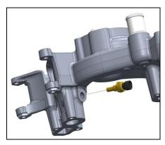
Install original temperature sensor removed from the LT water pump manifold. Torque to 15 ft/lb.
