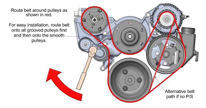
After routing the belt, use a 1/2" square drive wrench to pull the tensioner all the way down and work the belt on from the rear.
