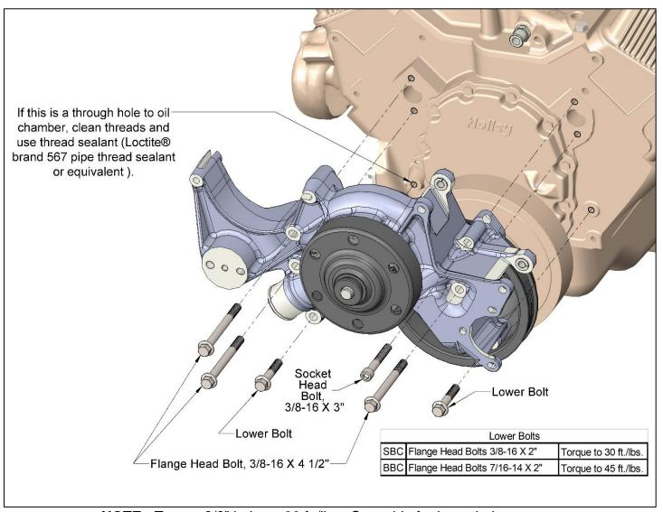
**NOTE:** Torque 3/8" bolts to 30 ft./lbs. See table for lower bolts torque.
