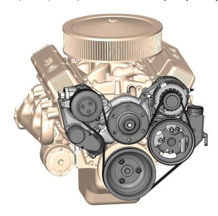
Holley's Mid-Mount complete accessory system has all accessories pulled in tighter than other accessory drives. Among the many features is the bracket-less assembly that actually mounts all accessories to the water pump directly.
