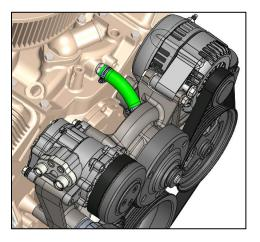
Thermostat bypass with standard-hose installation shown in green to the left. Hose and clamps not included.
