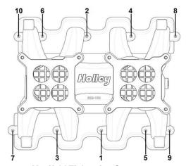
**Manifold Tightening Sequence**
