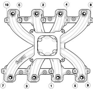
**Manifold Tightening Sequence**
