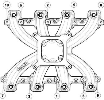
**Manifold Tightening Sequence**
