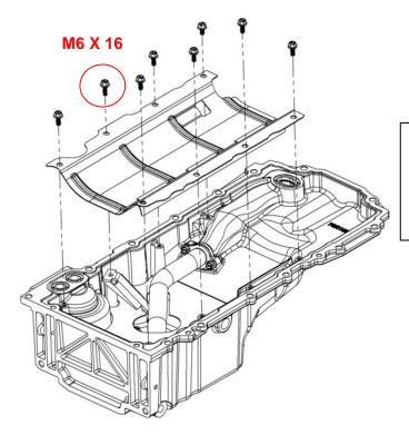
Install the windage tray. Apply a drop of blue Loctite® to the threads of the supplied (x7) M6 x 12 flange head bolts. Install the (x1) M6 x 16 flange head bolt in the location that also goes through the pickup tube bracket. Torque the bolts to 10 lb./ft.
