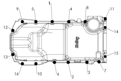
Torque: M8 bolts to 18 lb./feet. (bolts 1 through 13). M6 bolts to 106 lb./inch. (bolts 14 and 15).
