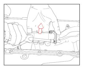
**IMPORTANT:** While the bolts are started, but still loose, lift the pickup tube. Tighten the two bolts while maintaining the lifted position. This process ensures proper clearance between the pickup inlet and the pan floor.
