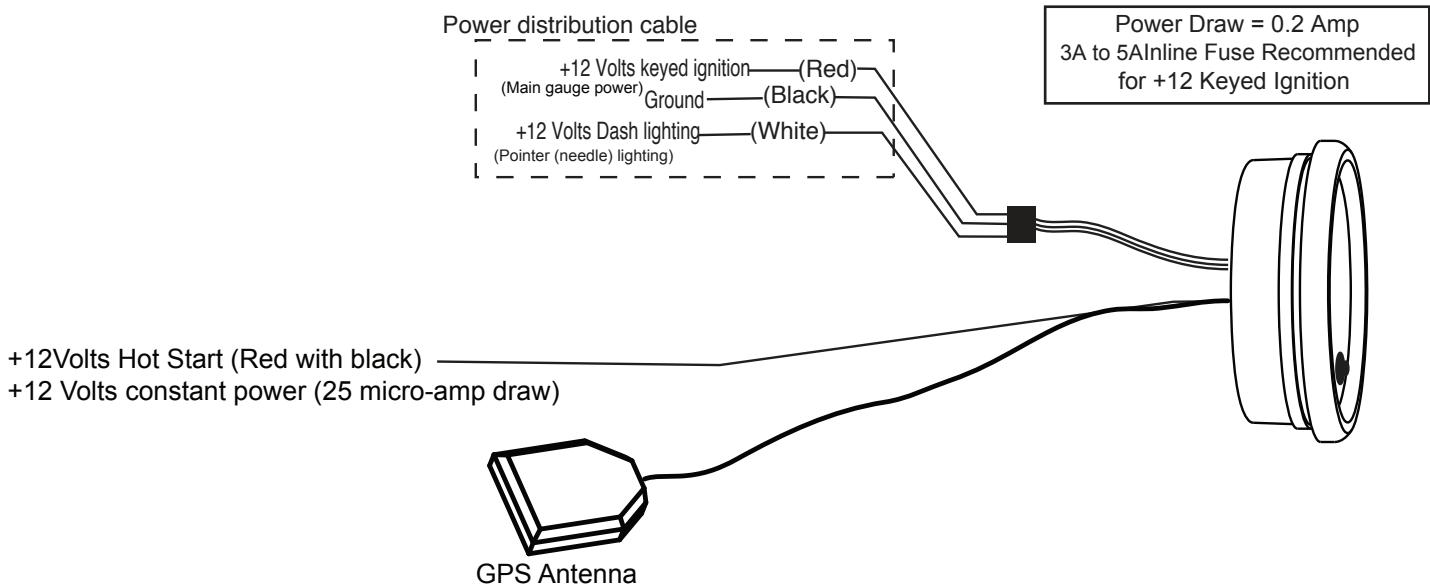
1. Connect speedometer power requirements as shown above.
