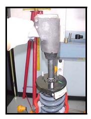
14) Reinstall the spring shock assembly in the same manner as removal. When installing the lower shock bolt make sure the hole lines up with the shock clevis. Make sure the threads start correctly by threading the bolt by hand. Once properly threaded fully tighten hardware.
