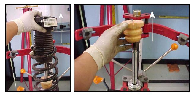
10) Place your new Hotchkis polyurethane bumpstop into the top hat boot assembly as shown in the picture.
