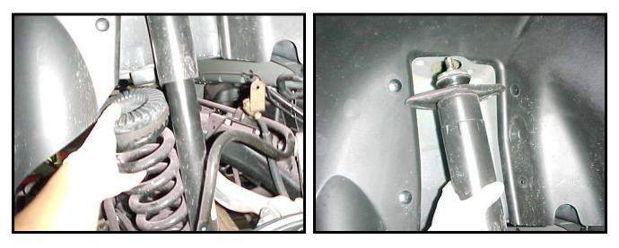
10) For each shock, unbolt the shaft nut using a 15mm socket. Remove the washer, top hat, and the boot to reveal the stock bumpstop. Replace the bumpstop with the provided Hotchkis polyurethane bumpstop in the same manner. Reassemble the shock. Fully tighten the shaft nut. Note: Daytona R/T Vehicles uses STOCK rear bumpstops.
