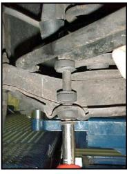
3) Turn the front wheels to point straight ahead. If you jacked up the front of the vehicle, you should now lower the vehicle so that the weight is on the front tires. Slide the stock bar towards the passenger side of the vehicle. The end of the sway bar should contact the rear edge of the brake drum preventing you from fully removing the sway bar.
