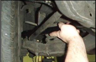
The leading end of the bar should eventually swing into the slot in the frame on the driver's side of the vehicle. The bar will be free moving, but in the proper orientation in the vehicle.
