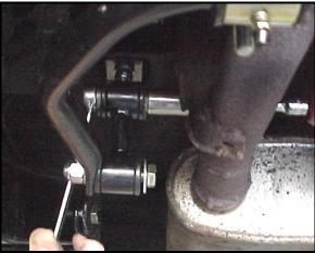
12) Check that all hardware is tight. Use the caps provided to cover the zerk fittings and you're done installing the Hotchkis rear sway bar!
