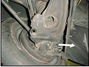
4) Move the sway bar end towards the rear on the passenger side of the vehicle until the opposite end of the bar clears the slot in the frame on the driver's side.
