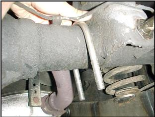
3) Use the grease pack provided to apply a heavy coat of grease to the inside of the sway bar bushings. Place the bushings over the bar. The split in the bushings should face towards the rear of the vehicle with the bar installed. Push the brackets over the sway bar bushings.
