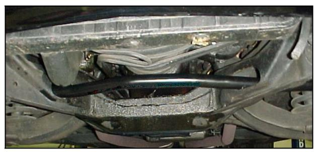
8) Use the grease pack provided to put a heavy coat of grease on the inside of the sway bar bushings. Place the bushings over the bar with the cut in the bushing towards the rear of the vehicle. Push the bushing retainer brackets into place on the bar and bolt them into place <u>using</u> the stock mounting hardware in the front holes only. **Do not** tighten the stock hardware.
