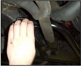
7) Slide the end of the Hotchkis bar between the coil spring and the brake drum in the same fashion as was used to remove the stock bar.
