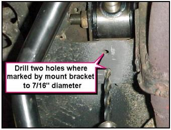
Drill out the holes for the brackets to 7/16" diameter. To accurately determine the location of the holes the end links must not be loose enough to move left or right. Make certain the axle is at its normal driving height for an accurate fit.
