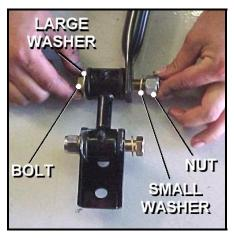
The large washer should be used to contact bushing surfaces and the small washer should be used to contact metal surfaces. This prevents the bolt from pulling through the bushing. You will have 2 large washers and 2 small washers left over. This is extra hardware and may be discarded.
