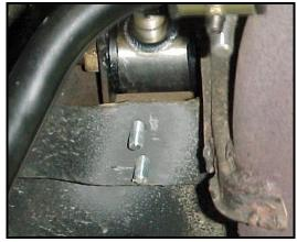
10) Unbolt the bracket from the end link. Hold the bracket back up in position to the bolts hanging from the frame. Use the nylock nuts included to hold the bracket on the bolts. Tighten the hardware holding the bracket to the frame. Torque the nuts to 80 ft/lbs.
