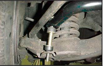
10) With the final position of the bar now determined, you will need a scribe or some other tool to mark with. Mark the center position of the holes for the rear side of the bracket. Remove the brackets, bushings, end links, and stock hardware. Drill the existing front mount hole out to a 7/16" diameter and drill a new rear mount hole at the same size where you marked the frame.
