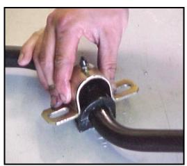
4) Use the grease provided to apply a heavy coat of grease to the sides of the bushings on the "dog bone" end links. Attach the mounting brackets to the end links using **hardware kit #T1712**. Attach the other end of the links to the sway bar. Leave the attaching hardware loose.
