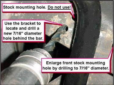
11) Use the 3/8" bolts from **hardware kit #1735** to attach the Hotchkis bar. Drop the bolts down through the drilled out holes in the frame. Start the washers and nylock nuts onto the ends of the bolts. You will use only four of each nut, washer and bolt. <u>DO NOT THROW THE EXTRA HARDWARE AWAY</u>, as it is used for the rear sway bar. Torque the hardware to 35 ft/lbs.
