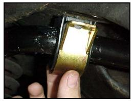
9) With the brackets in place, install the new end links included in the Hotchkis kit at each end of the bar to establish the proper fit of the front bar. The vehicle weight should be on the front wheels to establish the proper ride position of the sway bar in the vehicle.
