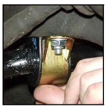
12) Re-place the end links removed in step 10 and tighten them into place. Tighten the end links until the nut meets slightly stiff resistance. The bushings will have a slight bulge when tight.
