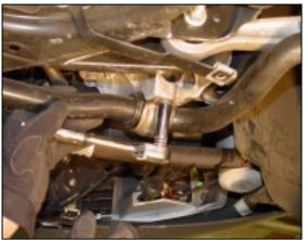
5/ Apply a quarter tube of grease to each inner portion of the two new front bushings and attach to HSport bar against the outside of the washers on the bar. Slip the new brackets over the bushings.
