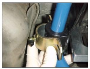
11/ Now, install the last 4 bushing bracket bolts and washers using the 13mm wrench and tighten. Remember, the black bracket is slotted so if all hardware is loose enough, you will be able to thread the bushing bracket bolts through the sub-frame and into the aluminum.
