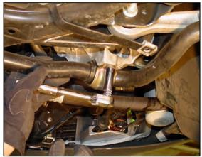
5/ Apply grease to each inner-channeled portion of the two new front bushings and attach to HSport bar against the outside of the washers on the bar. Slip the new brackets over the bushings.
