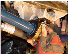
7/ Re-install the bracket nuts and tighten. *Use a small portion of blue thread-locker on the end-link bolts*, re-install and tighten well. \*\*Note\*\* If vehicle is raised using jack stands or other, the bar end and the end link may not align properly. Lower vehicle so that front suspension is not at full droop and ends will align. Be sure to thread end link bolt by hand at first to prevent cross-threading.
