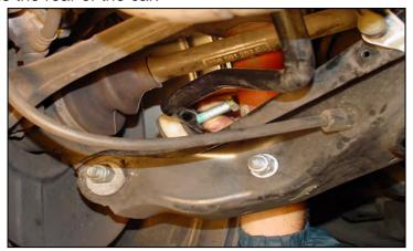
6/ As you begin to remove the bar, gently free each end from the end link. Now that the bar is free, slightly lower the exhaust by applying pressure to the tips just enough to remove the bar. (It will come out, be patient)
