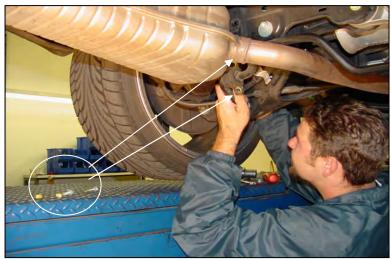
5/ Remove the two end link bolts and nuts (16mm wrench) which attach the bar ends to the end links and save them. To clear the shocks with the bolts, pull the bar towards the rear of the car.
