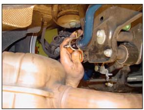
9/ Re-install the end link bolts (using the supplied 10mm washers in between the nut and the end link head) and nuts and leave loose. Secure the bushing brackets, using the supplied 8mm washers in between the nuts and the slots of the bushing brackets. Tighten the four bracket bolts, then tighten the end link bolts.
