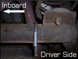
Next, apply the provided lube on the inside surface of the polyrethane bushings. Pop the bushings onto the sway bar. Slide the bushing brackets onto the bushings.
