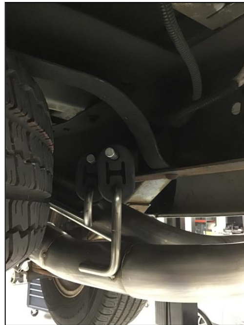
Figure 2 Rear tailpipe hanger to frame
