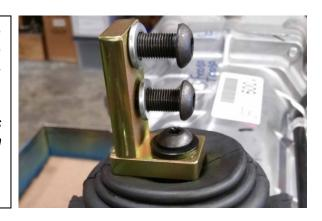
Attach the Chrome Hurst shift handle to the lower stub stick using the supplied hardware. Reinstall the shift boot and factory console. If you are using a properly designed crossmember and your car is in good condition (no floor sag, stock height sub-frame mounts that are not worn, and properly aligned sub-frame), there will be no modifications required to your floorboard or console when using this shifter.
