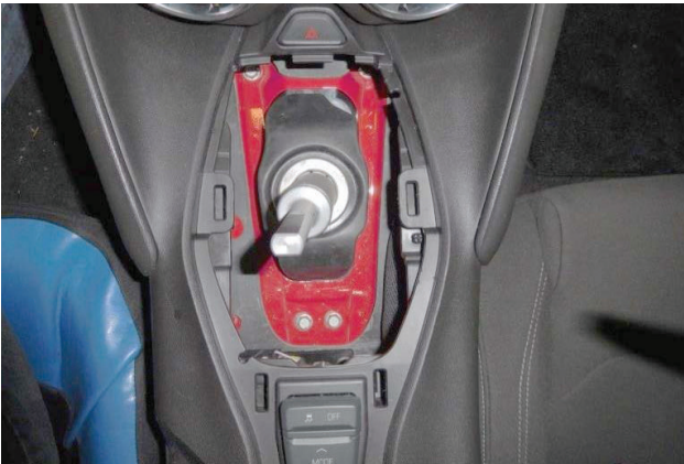
7. Remove (x4) bolts attaching rubber boot to transmission tunnel.
