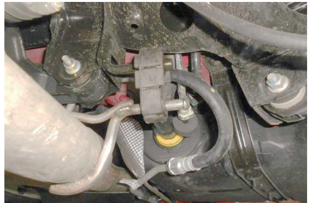
11. Remove forward isolators from exhaust system on left and right side.
