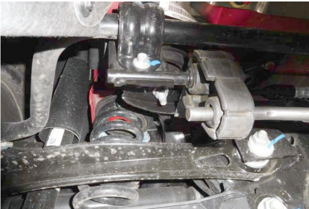
13. Remove mid hangers from left and right side of exhaust, then remove exhaust system completely.
