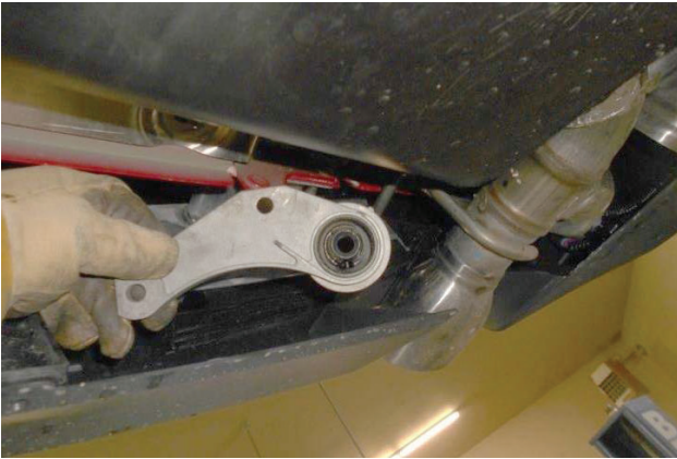
12. Remove (x2) nuts and hangers attached on left and right side at rear of vehicle.
