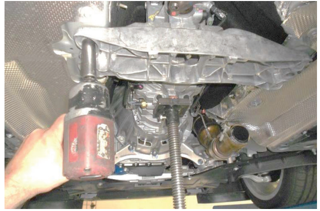
21. Support transmission then remove (x4) 15mm bolts from transmission cross member.
