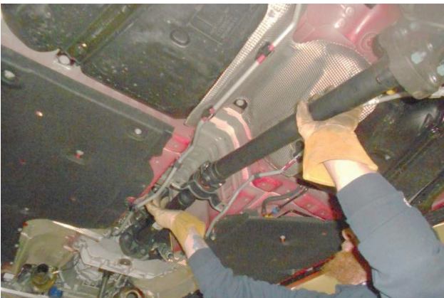
20. Remove drive shaft by squeezing it together in order to clear transmission and differential flange.
