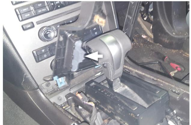
5. Unplug connector at front of console then remove upper console.
