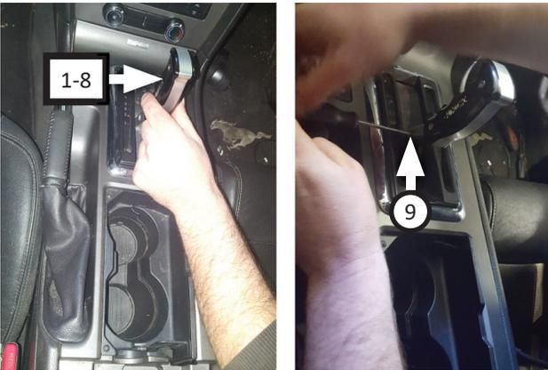
12. Install assembled **shifter (1-8)** and secure it in place with (x2) **screws (9)** as shown.
