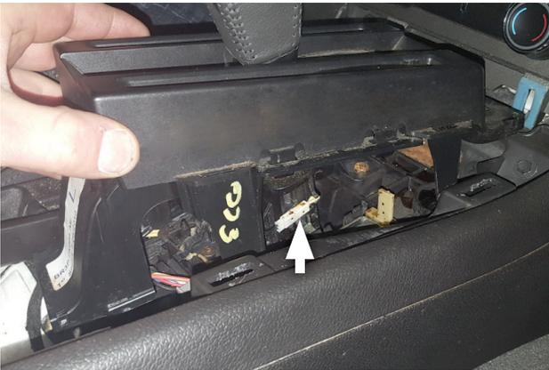
7. Disconnect (x4) tabs around base of shifter then unplug shifter wire underneath.
