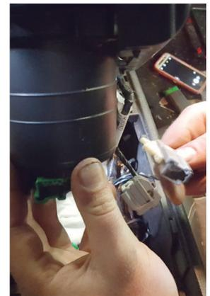
4. Unplug connectors and detach connector from bottom of console.
