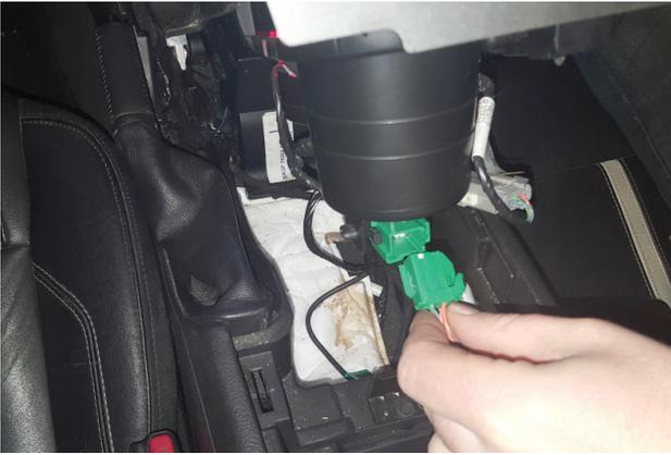
11. Replug connectors (unplugged step 4) into bottom of console, then press console down back into place.
