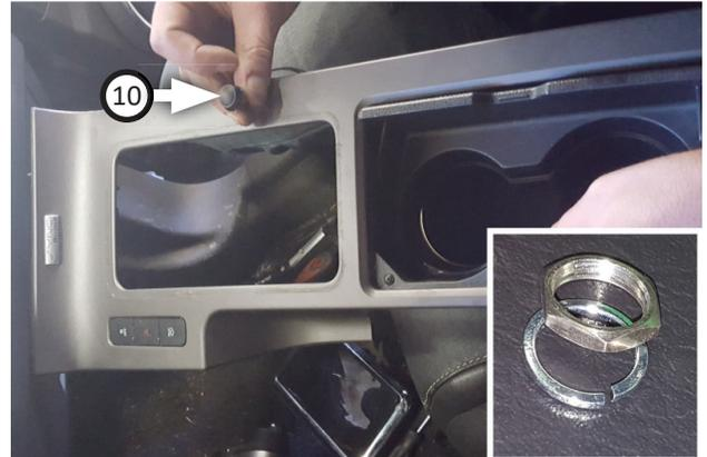
9. Choose install location (somewhere that wiring reaches shifter) then drill a  $1\frac{5}{32}$ " hole. Remove nut and lock washer from assembly, then pull switch wiring through hole until button is flush with console wall. Use nut and lock washer to secure button in place.
