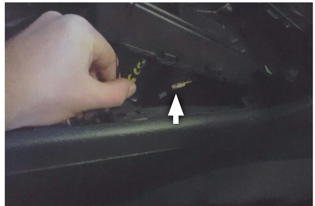
10. Pull shifter base up then plug push button switch wiring in on passenger side. Re-install top portion of shifter to base.
