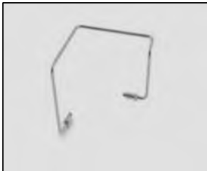
S. Steel Brake Line To Master Cylinder
