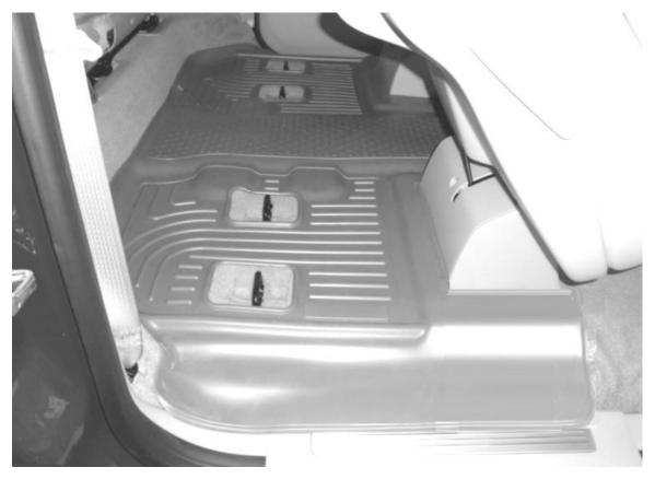
NOTE SEAT ATTACHES TO FLOOR THROUGH LINER
