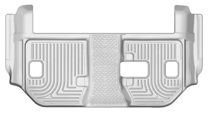
BEFORE ATTEMPTING TO INSTALL YOUR LINER, FIRST FLIP/FOLD YOUR SECOND ROW SEATS FORWARD TO EXPOSE THE 3<sup>RD</sup> ROW FLOOR PAN. WITH THIS DONE YOU CAN POSITION THE LINER IN THE FLOOR ORIENTED AS SHOWN ABOVE. NOTE THAT THE TWO DOOR EDGE TONGUE SECTIONS TUCK UNDER THE 2<sup>ND</sup> SEAT LINER.
