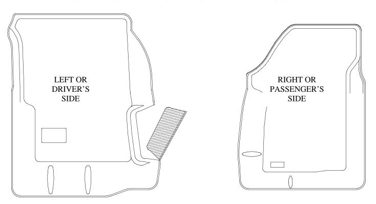
IF YOUR SUPERDUTY IS EQUIPPED WITH A MANUAL TRANSFER CASE SHIFTER, YOU WILL NEED TO TRIM YOUR MAT AS SHOWN ABOVE. TRIM AWAY THE RAISED AREA ON YOUR LINER. A UTILITY KNIFE WORKS WELL FOR TRIMMING.
