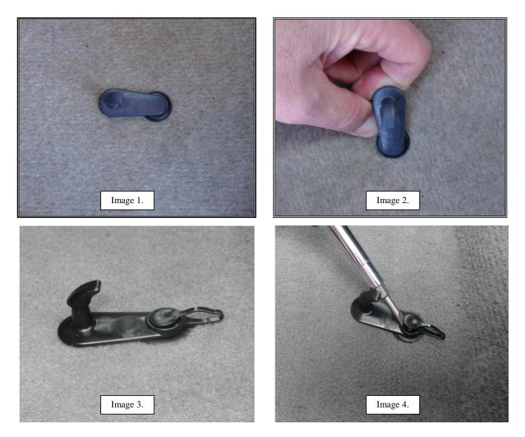
2) WITH THE FACTORY CLIPS REMOVED, UNSCREW THE TWO HALVES OF THE HUSKY<sup>®</sup> RETAINING CLIP AND INSERT THE BOTTOM HALF INTO THE EXISTING FACTORY GROMMETS LOCATION AS SHOWN BELOW IN IMAGE 4 AND IMAGE 5. THE BOTTOM PORTION WILL "SNAP" SECURELY INTO THE FACTORY GROMMET LOCATION. RETAIN THE TOP HALF OF THE CLIP FOR LATER INSTALLATION.
