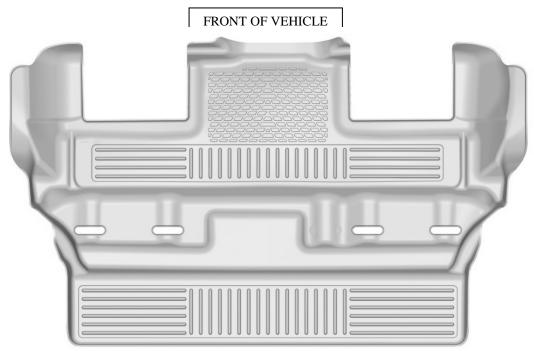
BEFORE ATTEMPTING TO INSTALL YOUR LINER, FIRST FLIP/FOLD YOUR SECOND ROW BUCKET SEATS FORWARD TO EXPOSE THE  $3^{RD}$  ROW FLOOR PAN. WITH THIS DONE YOU CAN POSITION THE LINER IN THE FLOOR ORIENTED AS SHOWN ABOVE. THE "TONGUE" AREA PROVIDES COVERAGE BETWEEN THE  $2^{ND}$  ROW BUCKET SEATS AND TUCKS UNDER THE REAR EDGE OF YOUR  $2^{ND}$  SEAT LINER.
