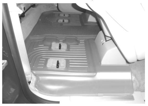
NOTE SEAT ATTACHES TO FLOOR THROUGH LINER
