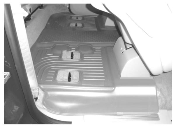
NOTE SEAT ATTACHES TO FLOOR THROUGH LINER
