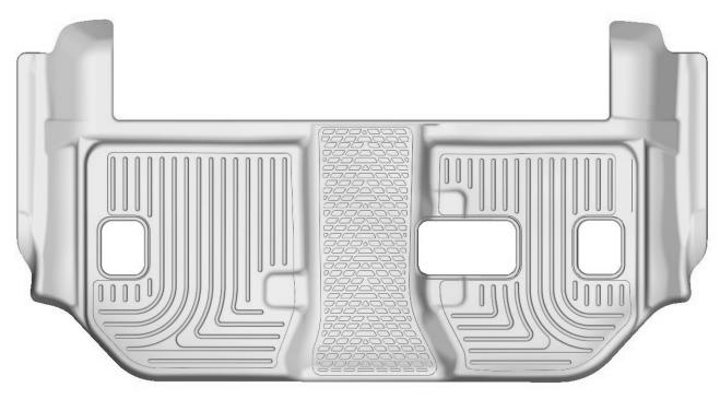
BEFORE ATTEMPTING TO INSTALL YOUR LINER, FIRST FLIP/FOLD YOUR SECOND ROW SEATS FORWARD TO EXPOSE THE 3<sup>RD</sup> ROW FLOOR PAN. WITH THIS DONE YOU CAN POSITION THE LINER IN THE FLOOR ORIENTED AS SHOWN ABOVE.
