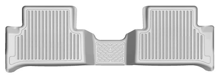
TO EASE INSTALLATION OF YOUR COLORADO / CANYON SECOND SEAT LINER, MOVE THE FRONT SEATS TO THEIR MOST FORWARD POSITIONS. WITH THIS DONE, INSERT LINER IN VEHICLE ANGLING THEM SO THAT THE FRONT EDGE OF THE LINER IS SEATED INTO PLACE FIRST, THEN LOWER THE REAR OF THE LINER. ONCE THE LINER IS INSTALLED, REPOSITION THE FRONT SEATS AS DESIRED.
