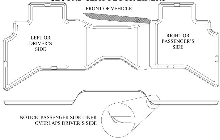
NOTE: IF YOUR DODGE RAM QUAD CAB TRUCK HAS FRONT BUCKET SEATS WITH THE CONSOLE OPTION, YOU WILL NEED TO TRIM YOUR LINER AS SHOWN ABOVE (SEE HATCHED AREA). TRIM ALONG THE BACK EDGE OF THE RAISED RIB (LEAVING THE RAISED RIB ATTACHED TO THE PART) AND THEY FOLLOWING THE MOLDED GROOVE DOWN THE HUMP. A UTILITY KNIFE OR HEAVY SHEARS WORK WELL FOR TRIMMING.
