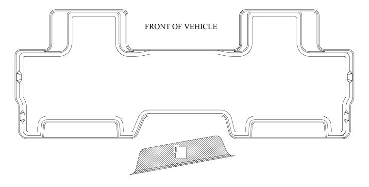
NAVIGATOR OWNERS WHOSE VEHICLES ARE EQUIPPED WITH THE SECOND SEAT CONSOLE WILL NEED TO TRIM THEIR LINER TO ALLOW FOR THE CORRECT FIT. TO TRIM, SIMPLY REMOVE THE TREADPLATED AREA FROM THE RAISED CENTER PORITON OF THE LINER (SEE AREA "1" ABOVE SHOWN CROSS HATCHED). USE THE EDGE OF THE TREAD AS YOUR TRIMMING GUIDE (SEE PHOTOS ON BACK). A UTILITY KNIFE OR HEAVY SHEARS WORK WELL FOR TRIMMING.
