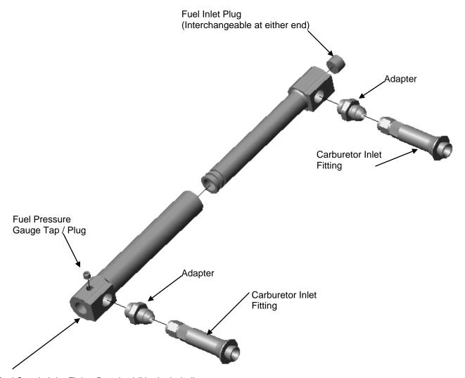
Fuel Supply Inlet Fitting Required (Not Included)
