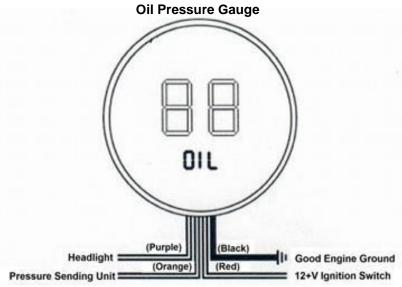
*Ground* - **Black** Connect directly to an engine ground such as the engine block. For the most accurate readings, connect to the same ground as that to which the sending unit is attached.
