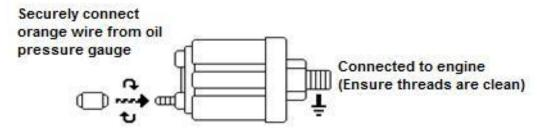
**Make sure** that the connection between the oil pressure sensor and the engine is clean and **does not** have thread tape or any other sealants on the threads. This provides a stable ground for the sensor and will not function if it is inhibited.
