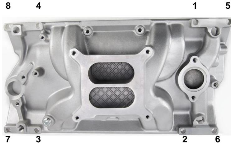
6. Install the thermostat, gasket, and thermostat housing. Be sure that the thermostat housing is in good condition and has been cleaned of any old gasket material. If the mounting flange on the thermostat housing is not flat or is damaged, replace it before continuing.
