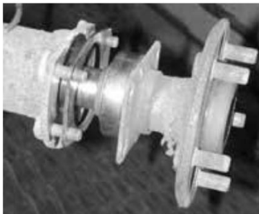
Installation of Spacer Plate
