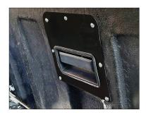
10. Place assembled relocator bracket and handle into the hole, double-check mounting hole marks, then drill and install mounting screws.
