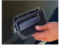
2. Carefuly remove the handle from its original position making sure to un-clip the attached rods.
