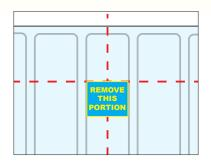
Using a straight edge, mark a square <sup>1</sup>/<sub>4</sub> in. inside of the mounting hole marks. This is the area to be cut out.
