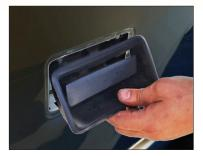
Carefuly remove the handle from its original position making sure to un-clip the attached rods.
