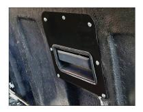
Place assembled relocator bracket and handle into the hole, double-check mounting hole marks, then drill and install mounting screws.
