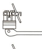
Clamp the tool in a suitable bench mounted vice. Assemble the lever into the cam as shown. Loosen the clamping screw to allow the clamp to swing open.
