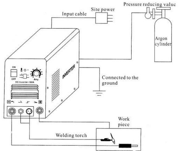
**Warning!** Before connecting operation please make sure all the power is turned off. First, connect the welding cable and ground cable to the machine, make sure they are firmly connected and then put the power plug to the power source.
