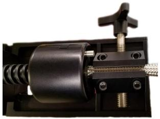
5. Turn Knob and press Button to release hose assembly.
