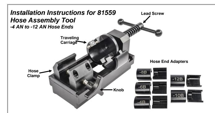
Clamp Hose Assembly Tool into vise. Turn Knob to open the Hose Clamp. Press button to open the Traveling Carriage.
