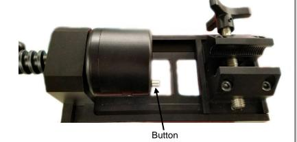
2. Place the desired Hose End Adapter into the Traveling Carriage. The larger of the two pieces, of the Hose End Adapter, will go into the bottom half of the Traveling Carriage. Measure the depth of the hose end to prevent over threading. Install the hose end into the Hose End Adapter as shown. Close the Traveling Carriage.
