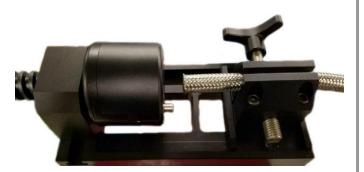
4. With the Traveling Carriage closed and the hose clamped in place begin rotating the Lead Screw until it cannot rotate any further.
