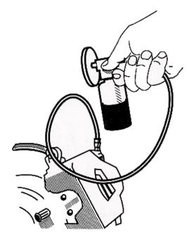
WARNING! Brake fluid is corrosive. Avoid contact with painted surfaces, clothing, skin and eyes. Wear eye protection. Follow vehicle manufacturer's sequence order for bleeding brake lines If you jack vehicle up, BE SURE TO USE JACK STANDS!
