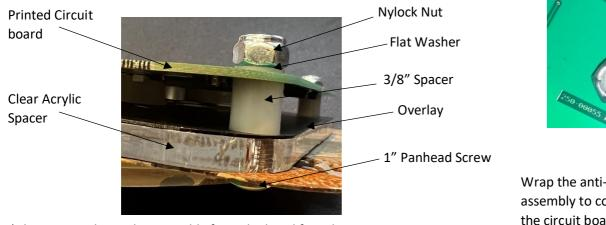
\*This picture shows the assembly from the bezel face down
