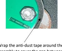
Wrap the anti-dust tape around the assembly to cover the gap between the circuit board and clear spacer
