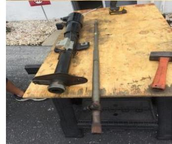
Cut steering column at 22 3/8" from the steering wheel as shown in pictures.
