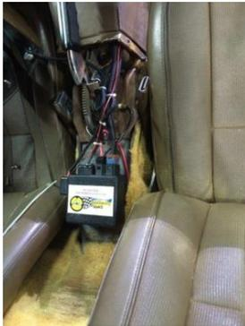
The wires will run inside the console, the power wire will go from front to back blue terminal and the torque sensor from back to front Delco pack and small red ignition wire from back to front as well.
