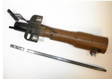
Then cut 3 1/2" of the steering shaft, the shaft will then slide into the 3/4" DD on the electric motor and tighten the two set screws.
