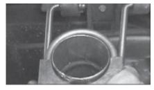
13. Install factory rear tail pipe rubber grommet on rear tail pipe hanger rod.
