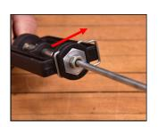
5) Secure the collet into position by sliding the locking spring into the closed position.
