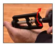
7) Rotate the lapping head back and forth in the flare until a clean seat is formed. Do not lap more than what is necessary.
