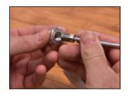
2) For the P-45, screw the fitting into the 3/16" collet for 3/16" tube and the 1/4" collet for 1/4"
