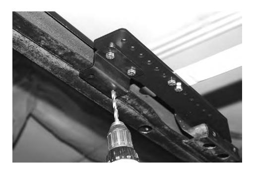
**SHORT SHELF only** - When using the extra bracket you will need to drill the mounting holes in the frame with a 25/64" drill bit. Install the 3/8"-16 x 1" bolts, flat washers and the 3/8"-16 nylon lock nuts.
