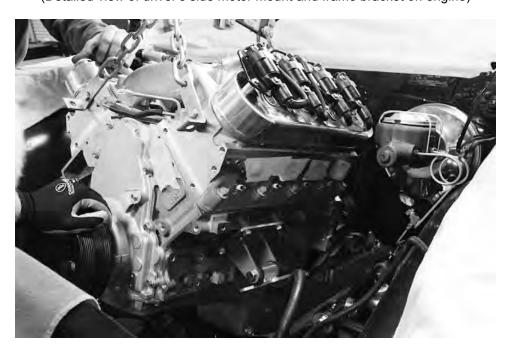
(Set the engine in place with each sides motor mount and frame bracket loosely on engine)
