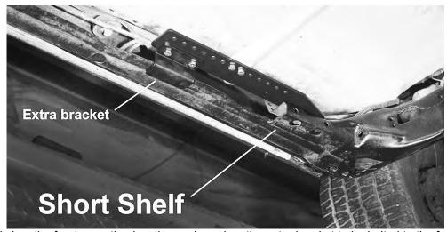
Short shelf only has the front mounting location and requires the extra bracket to be bolted to the frame.
