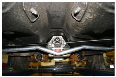
NOTE: You will need to have the existing driveshaft cut down to fit the new longer overdrive transmission or a custom driveshaft built.
